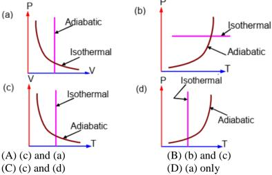
Ans:- (C) Pressure decreases with increase in volume, in both isothermal and adiabatic process. In adiabatic process, volume decreases and pressure increases with increase in temperature
