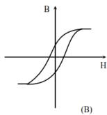
These materials are used to make magnets for electric generators, transformer core and electromagnet core.
