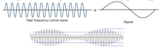
Amplitude modulated carrier wave
