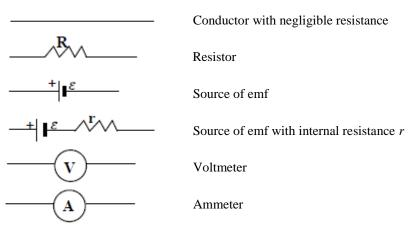
An important part of analyzing any electric circuit is drawing a schematic circuit diagram. We will use these symbols extensively in this chapter and the next. We usually assume that the wires that
